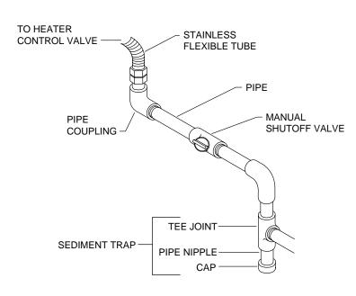
**IMPORTANT:** Loosen the pipe adapter on the flex tube before installing to the system piping.
